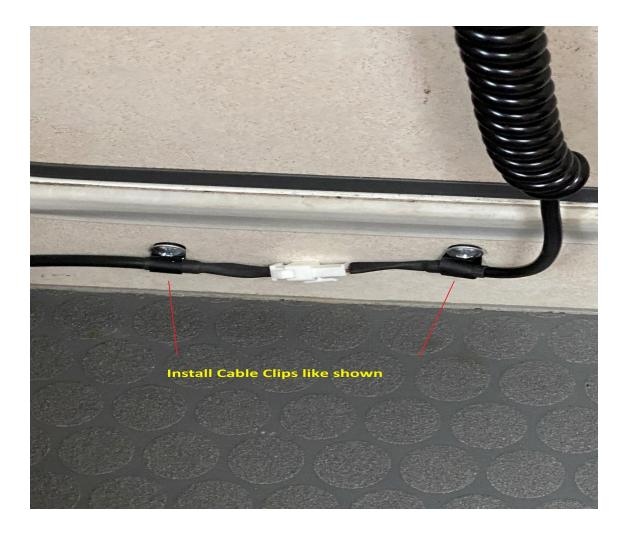
this will keep the cable from snagging when opening and closing door as it will expand on opening and return back to being coiled when in the closed position.
