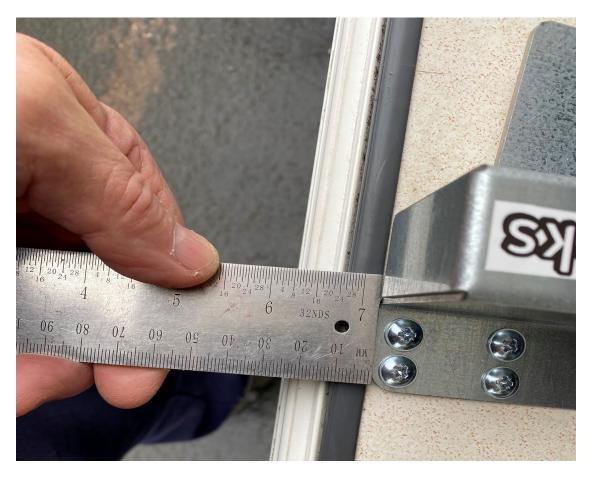
You may have to trim the inside door rubber so the lock can fully work without any restriction i.e. the moving parts of the lock should not be hindered in anyway.
